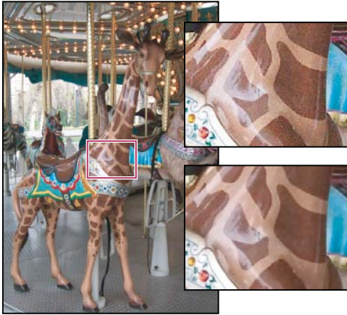
Moving the Luminance Smoothing slider to the right reduces grayscale noise, and moving the Color Noise Reduction slider to the right reduces chroma noise.
