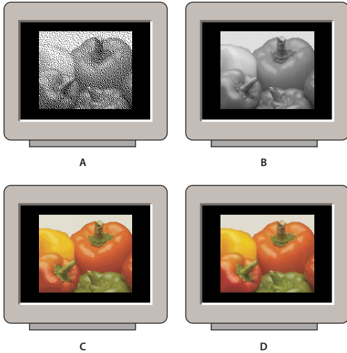
Pixel depth A. 1-bit (Bitmap) B. 8-bit (Grayscale) C. 8-bit (Indexed Color) D. 24-bit (RGB)
